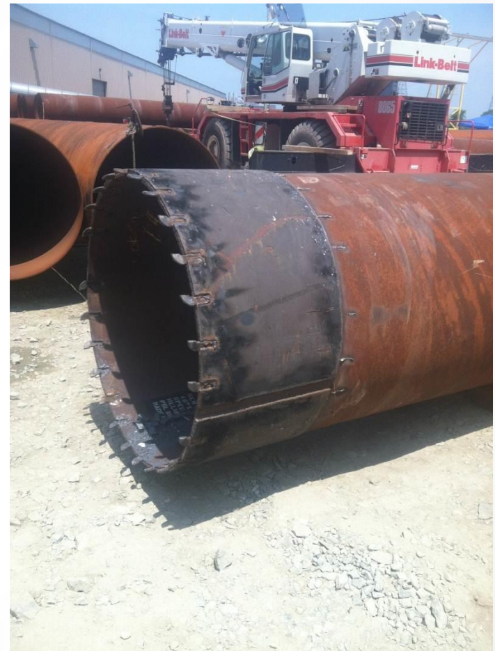
Cutting Teeth Welded to Casing
