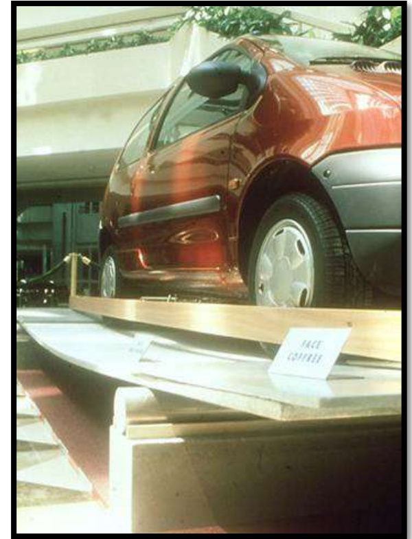
2,000 lb car on a 1 ¼ -inch sheet of Ductal®
